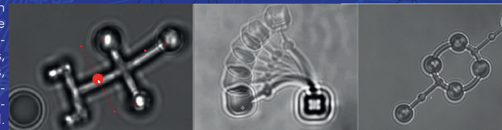
Various polymerized structures driven by laser traps. a) fork-like, b) elastic, c) rotating
