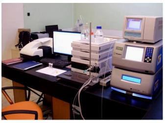
Fractionation of macromolecules or nanoparticles in asymmetric-flow field and subsequent simultaneous measurement of their concentration, size and molecular weight (Wyatt, USA). Extremely high resolution, for example, fig. to the left: BSA in form of a monomer, dimer, trimer, and higher associates.
